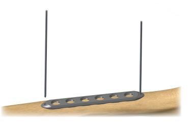
Conical and neutral ends of the 4 mm double drill sleeve both fit in the holes of the plate. Conical end provides ±15-degree angular freedom. Place the sleeve into the hole and perform drilling in the desired direction.
